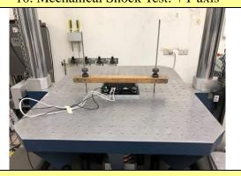
11. Mechanical Shock Test: -Y axis
